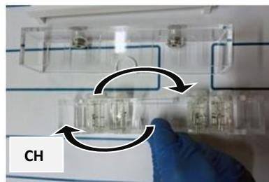
**4. REMOVE AND DISPOSE THE PLUGS** (place the cuvettes upright). Assemble MP4 (see p. 4) and place in its position on the mat (TC). Wait 5 minutes to retain the magnetic particles
