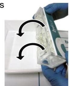
**8. Assemble the MP4 and place it in its position on the mat (TC) and wait 3 minutes** to retain the magnetic particles.
